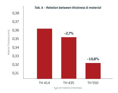
This optimization allows the end-users to save about two tons of raw materials out of one million pieces produced.
