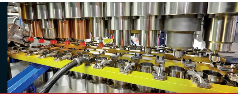
The innovative equipment of INVERNIZZI PRESSE allows to lower the costs for production of aerosol domes and spray cans Our machines are designed to work harder materials (from TH4335 to TH550) with or without coating that, in comparison with the standard ones used for the production of similar pieces, allows to obtain a finished product using a tinner plate, so literally employing less raw material.
